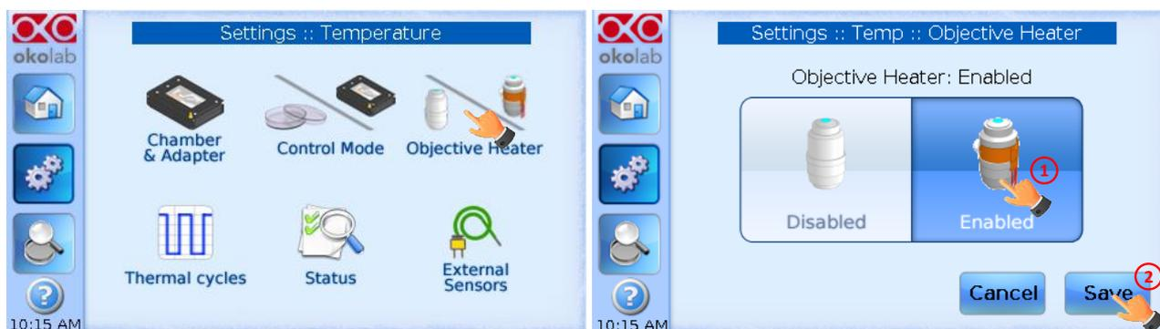
Figure 26. Objective Heater enabling.
