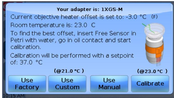
Figure 27. Objective Heater Calibration Page.
