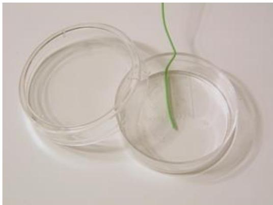
*Figure 44. Free Sensor attached on the internal base of the Petri Dish.*
