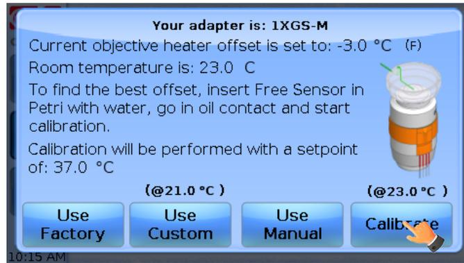
Figure 29. Objective Heater Self-Calibration Starting Message in Chamber Mode.
