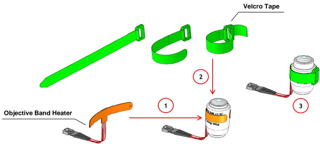
Figure 5. Objective Heater (OBJ-COLLAR ####) Assembly.
