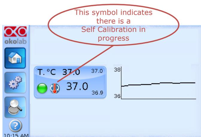
Figure 33. Homepage during Objective Heater Calibration.
