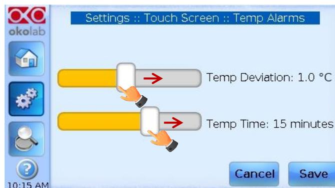
Figure 14. How to set the Deviation and Time Alarm.
