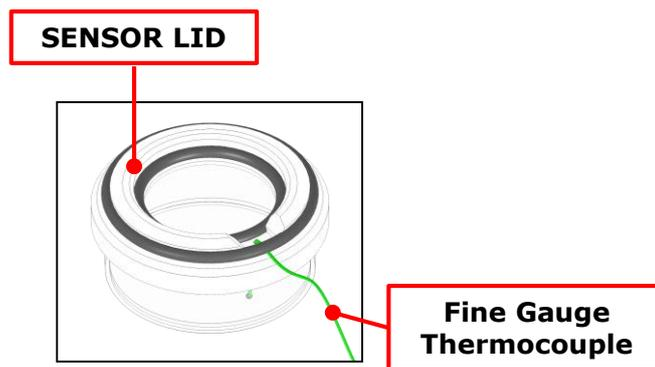
Figure 45. SENSOR LID-35. For 35 mm Petri-dish.
