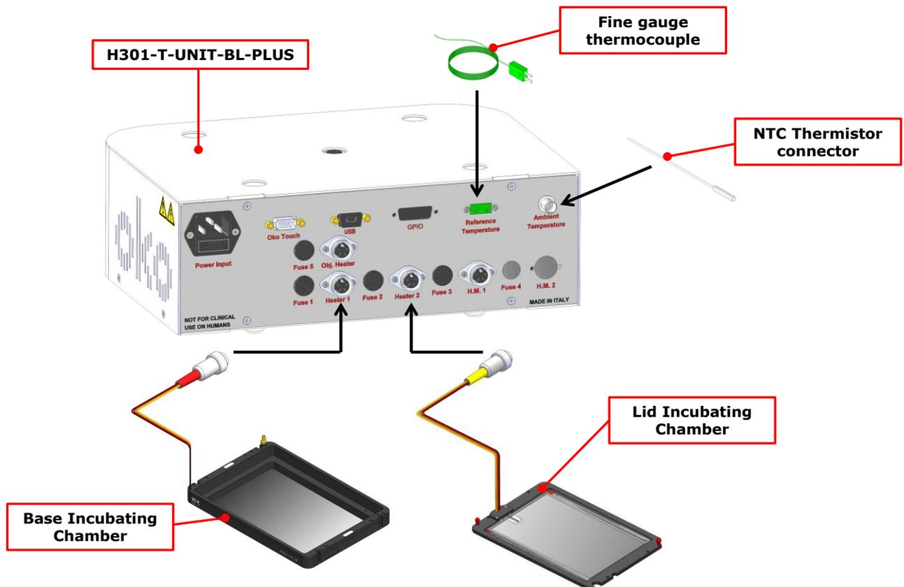
Figure 4. H301-T-BL-PLUS. Standard Connection.
