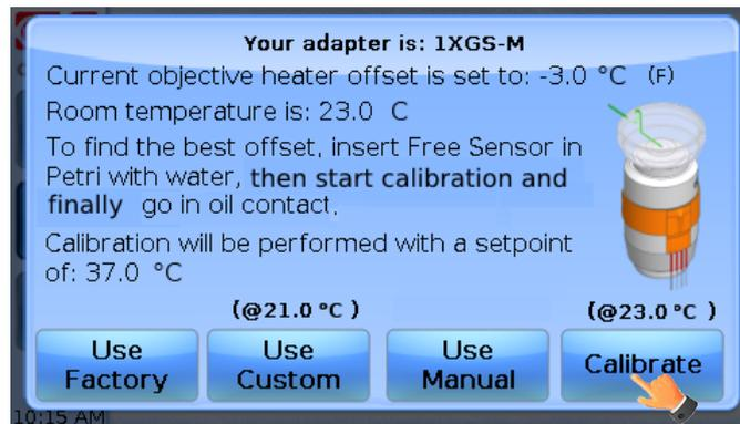
Figure 30. Objective Heater Self-Calibration Starting Message in Sample Mode.
