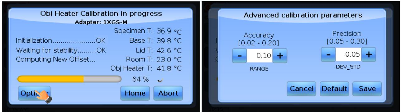
Figure 34. Objective Heater Self Calibration parameters.
