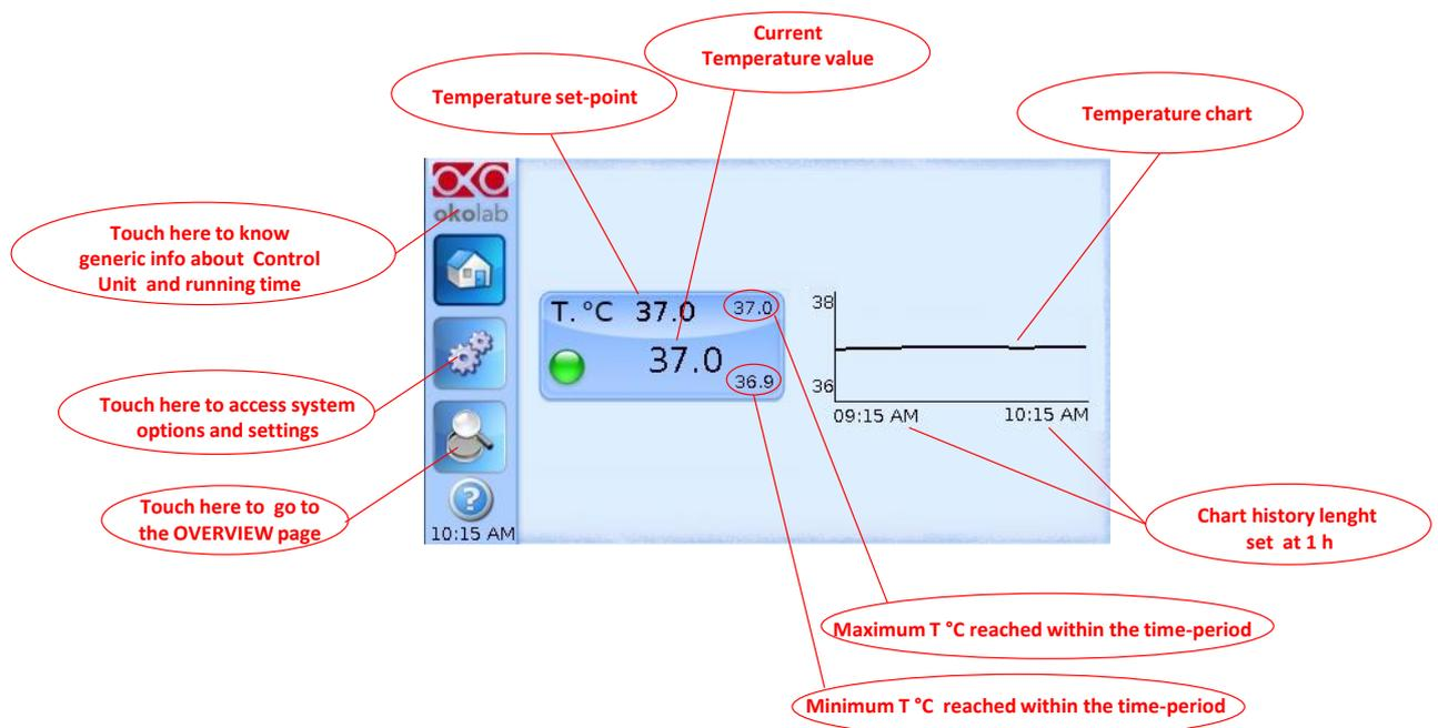
Figure 8. Homepage of the Control Unit Touch Screen Display.
