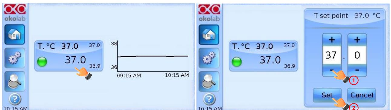
Figure 9. How to change the Temperature set point.
