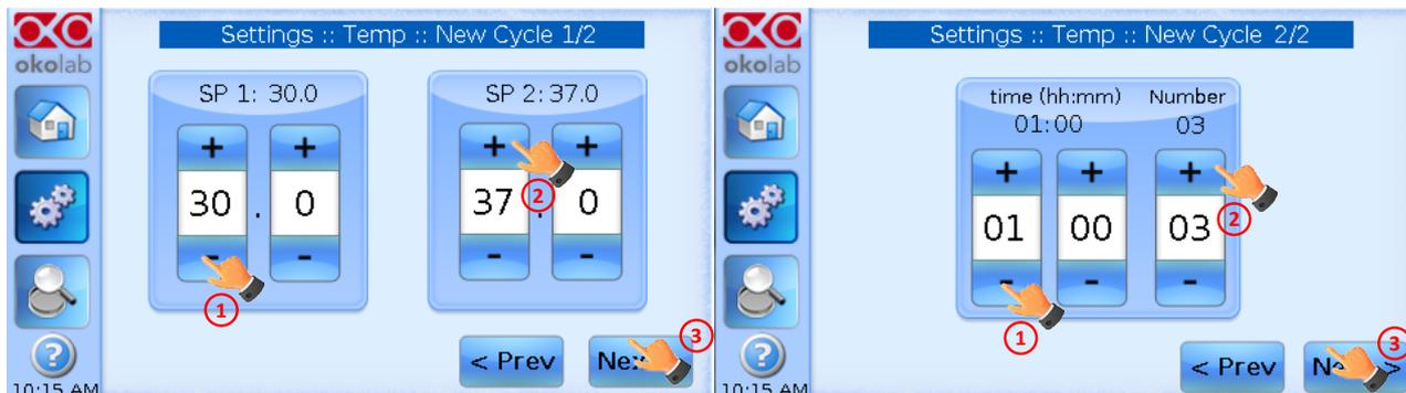
Figure 37. Thermal cycles settings.
